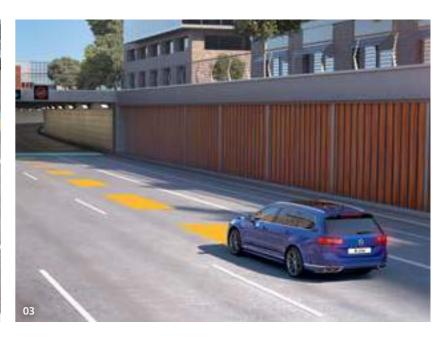
03 Adaptive Cruise Control (ACC) is a radar sensor controlled distance monitoring system that utilises a front mounted camera to set a distance to the vehicle in front and maintain it up to a predetermined set speed by automatically accelerating and braking as necessary. The system adds speed and cornering assistance by using information from the vehicle's navigation system if fitted. Standard on all models.
