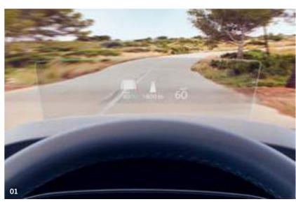
**01** The optional **Head-up Display**<sup>1</sup> presents driving information directly in your field of vision. Speed, traffic signs and information about the assistance systems, as well as warnings and navigation data are projected on to the high-quality retractable screen transparently displayed in front of the windscreen, enabling you to read everything clearly while keeping your focus on the road ahead. Optional on SE, SE Nav, SEL, R-Line, GTE, GTE Advance and Alltrack models.
